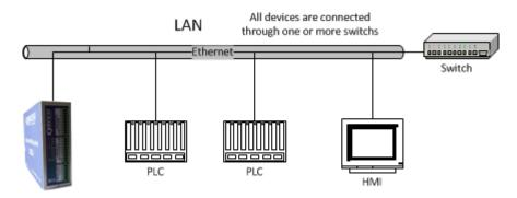
Config 4 - XL4 & PLC on own LAN segment, connected to each other by a switch
