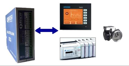
The DATRAN XL4 RTU has an Ethernet interface as standard, to maximise connectivity options. The Ethernet interface can be used for communications from the XL4 RTU to the DATRAN VI SCADA base station via ADSL or any internet connection providing communication options from anywhere in the world.
